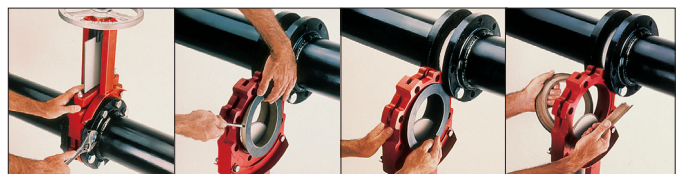
Cartridge slurry seat replacement process.
