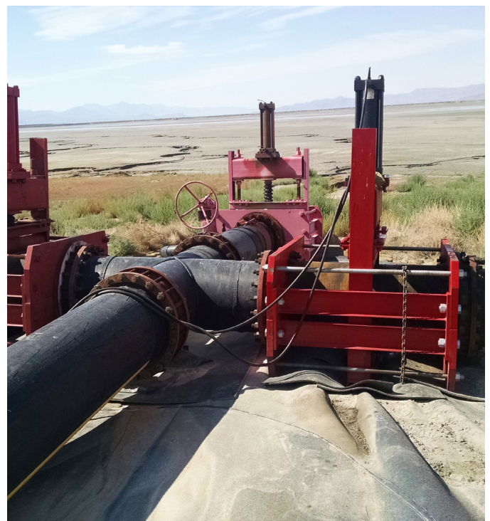
Open Frame Large-Diameter PCV - Series 5700 Control Pinch Valves used to control mine tailings.
