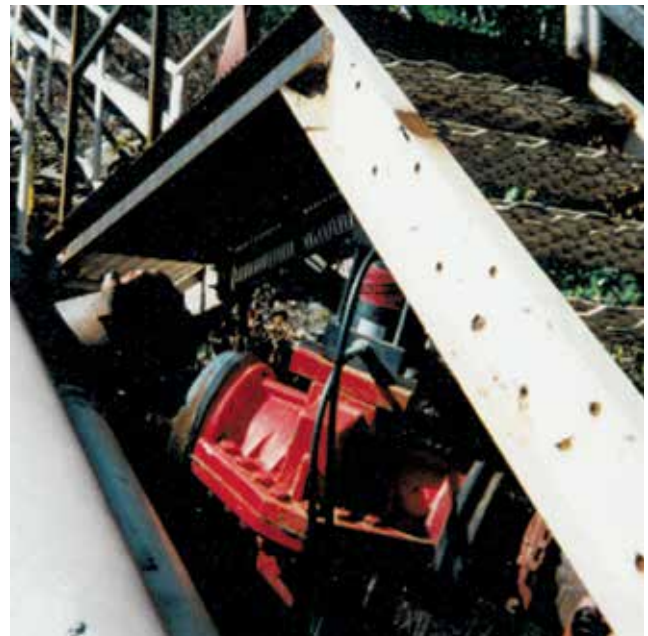
PCV - Series 9000 Hydraulic-Actuated Tailings Isolation Valve for 720 psi service at a mine.
